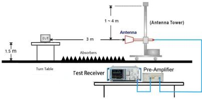
Above 1GHz Test Setup
