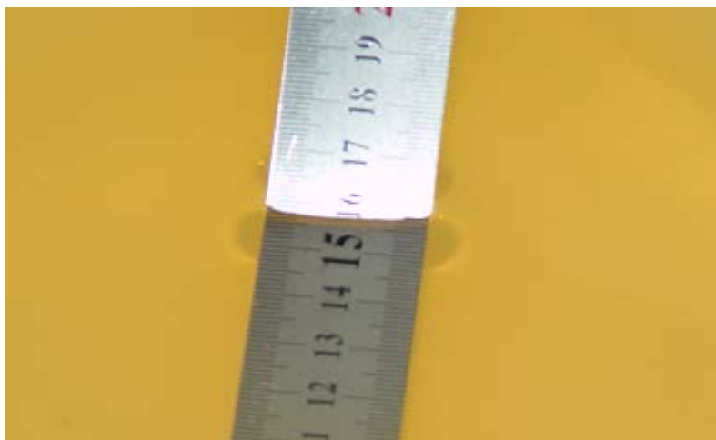
Liquid depth for SAR Measurement
