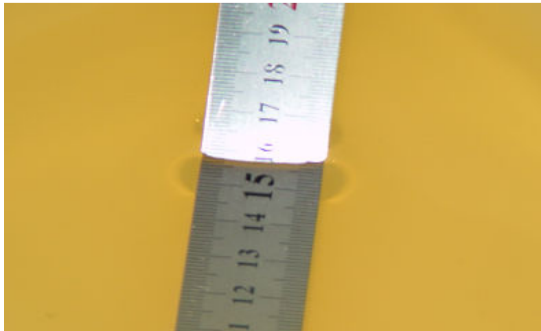
Liquid depth for SAR Measurement
