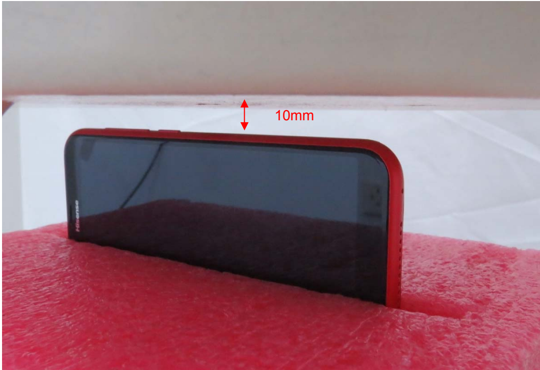
Picture 12: Right Side, the distance from handset to the bottom of the Phantom is 10mm
