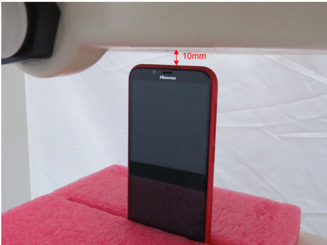
Picture 13: Top Side, the distance from handset to the bottom of the Phantom is 10mm
