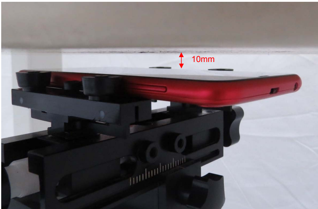
Picture 11: Front Side, the distance from handset to the bottom of the Phantom is 10mm
