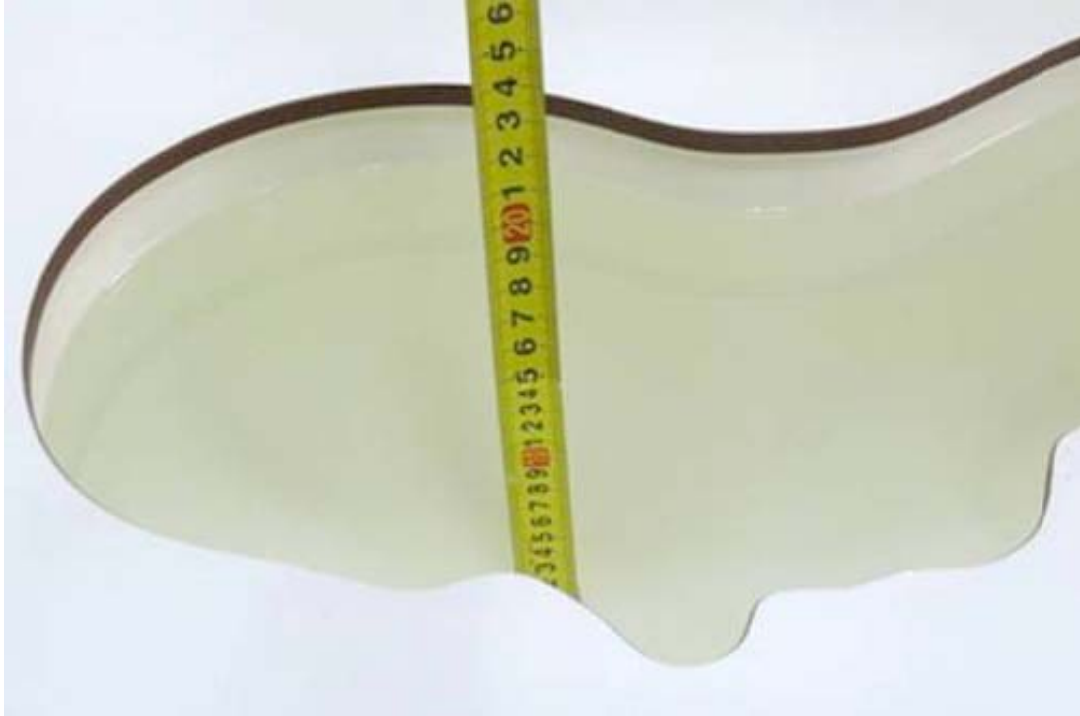
Picture 3: liquid depth in the head Phantom
