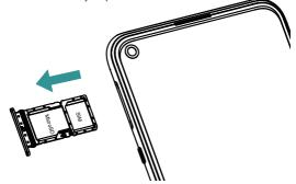
To eject SIM or MicroSD cards, insert your SIM eject pin into the small hole next to the card tray.
