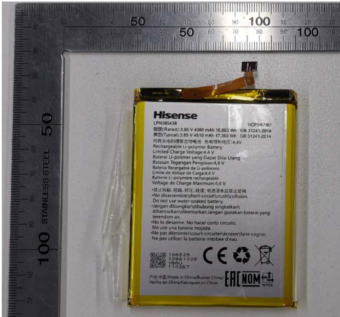
The battery view (ZHONGSHAN TIANMAO BATTERY CO., LTD.)
