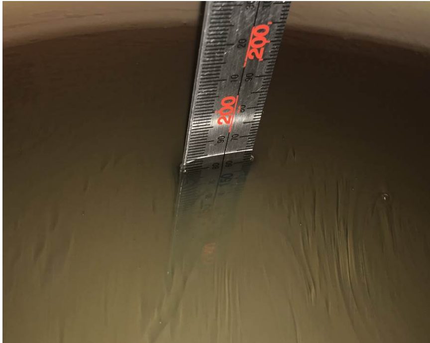
Liquid depth for SAR Measurement
