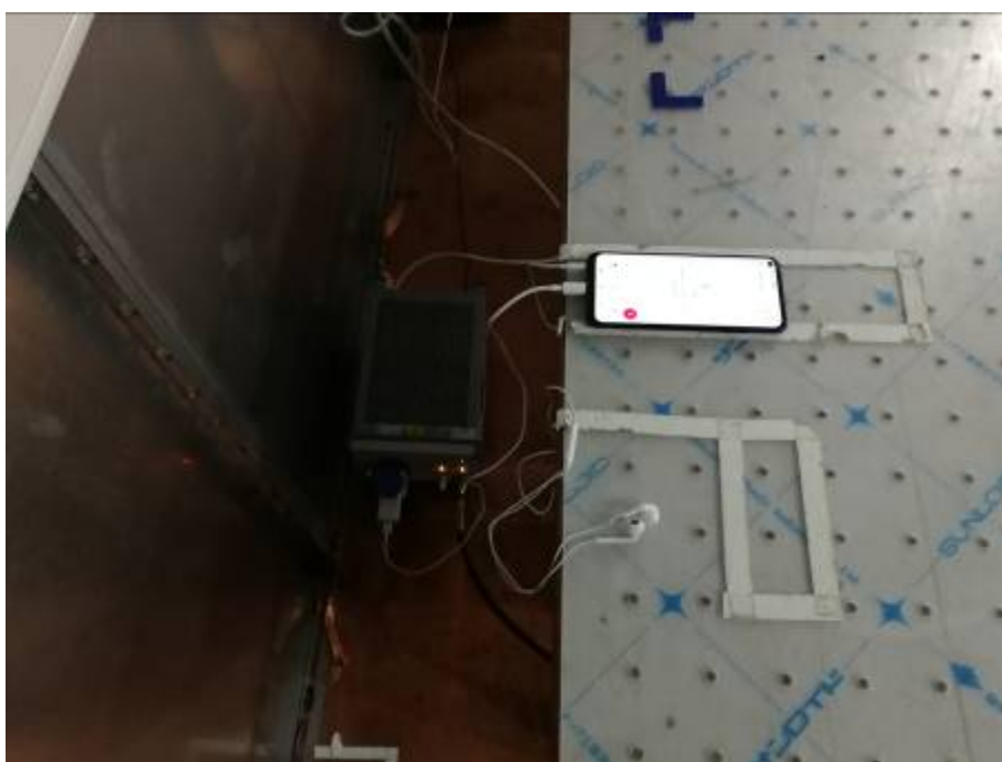
Conducted Emissions Test Setup (with charger)
