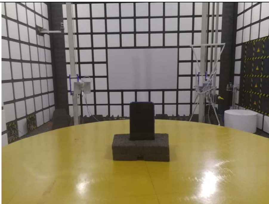
Spurious Radiated Emissions Test setup
