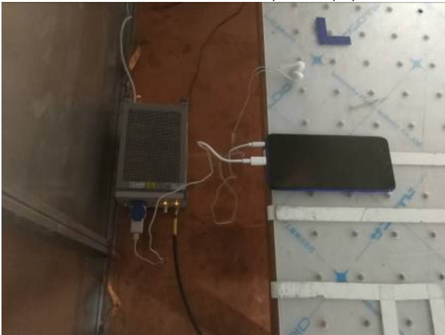
Conducted Emissions Test Setup (with charger)
