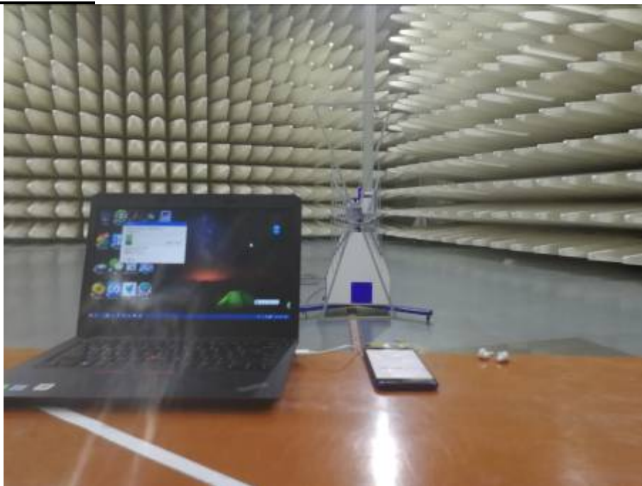
Radiated Emissions Test Setup (with laptop) (30-1000MHz)
