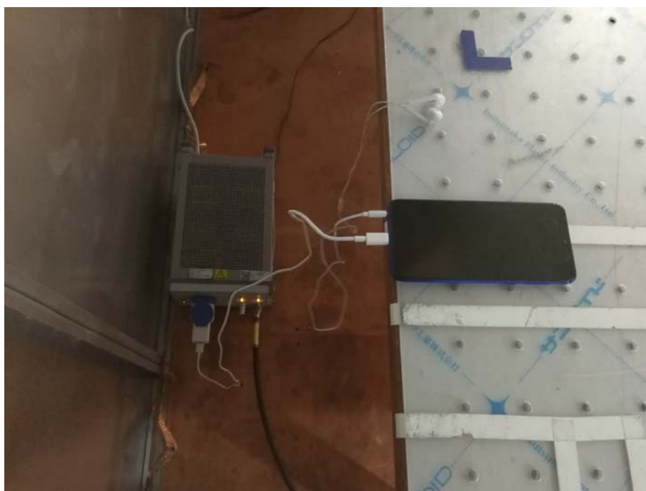
Conducted Emissions Test Setup (with charger)
