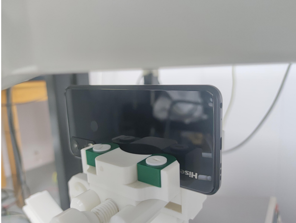
10mm body-worn Right Side Setup Photo (hotspot)
