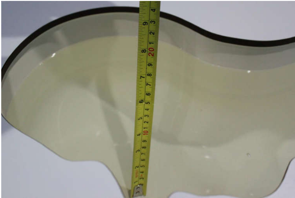
Picture 7-7: Liquid depth in the Head Phantom (5GHz)
