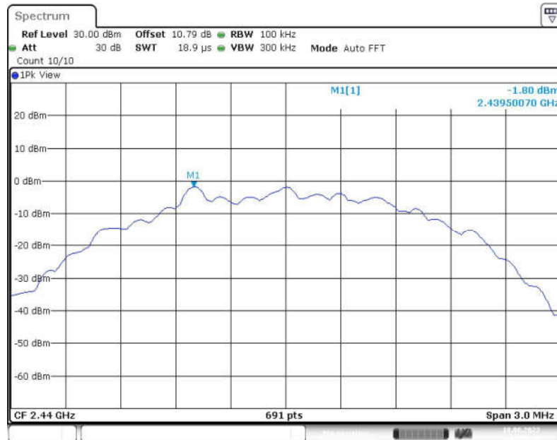
Fig.29 Conducted Spurious Emission (CH19, Center Frequency), LE 2M
