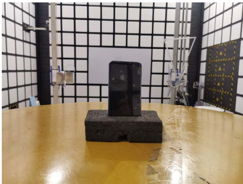
Spurious Radiated Emissions Test setup
