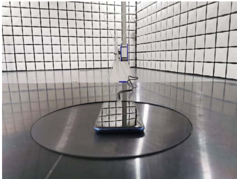
RF Conducted Test setup (BT/WIFI)
