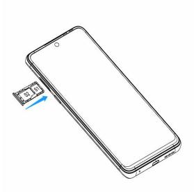
When inserting your card tray, make sure that the card tray is level and that the card is aligned correctly.
