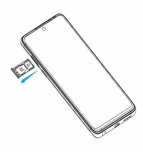
To eject SIM or MicroSD cards, insert your SIM eject pin into the small hole next to the card tray.
