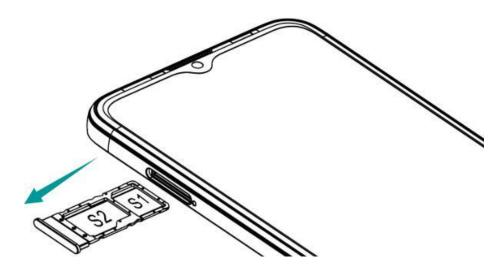
To eject SIM or MicroSD card, insert your SIM eject pin into the small hole next to the card tray.
