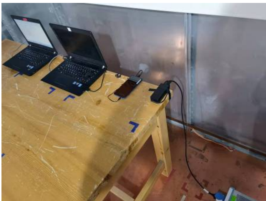
Conducted Emissions Test Setup (with laptop)
