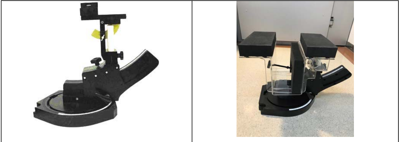
Device holder supplied by SPEAG
