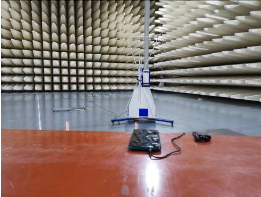
Radiated Emissions Test Setup (30-1000MHz)
