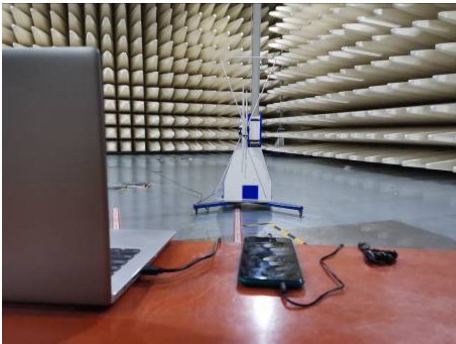
Radiated Emissions Test Setup (30-1000MHz)
