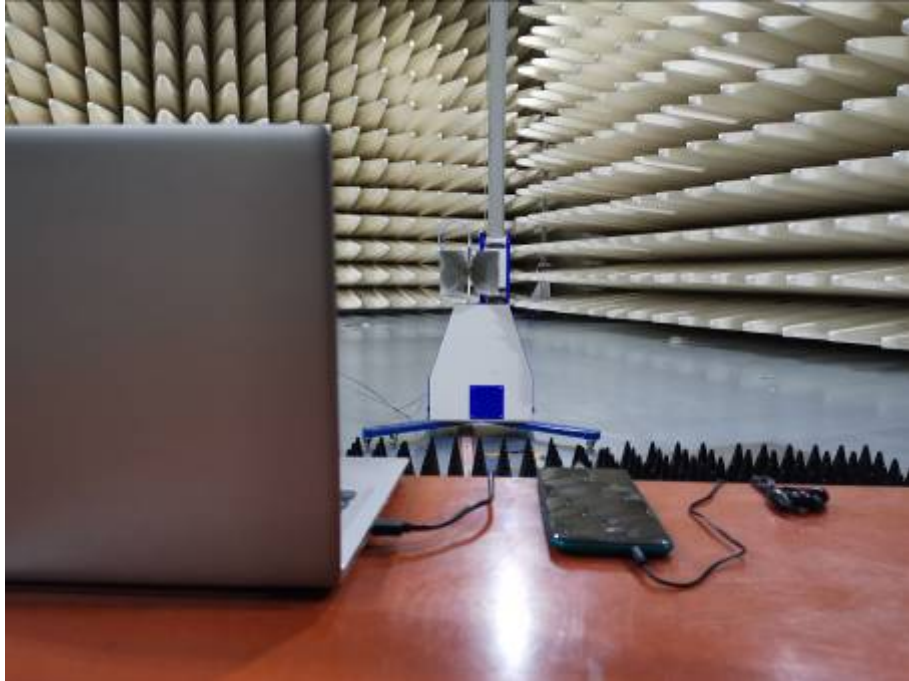
Radiated Emissions Test Setup (above 1GHz)
