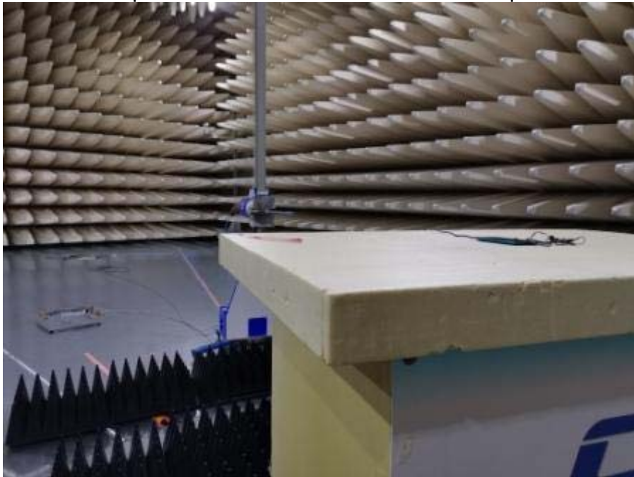
Spurious Radiated Emissions Test setup
