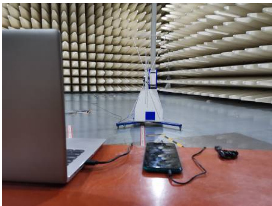
Radiated Emissions Test Setup (30-1000MHz)
