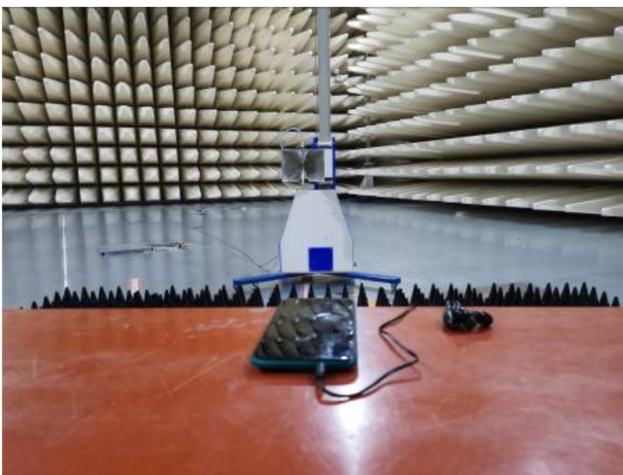
Radiated Emissions Test Setup (above1GHz)
