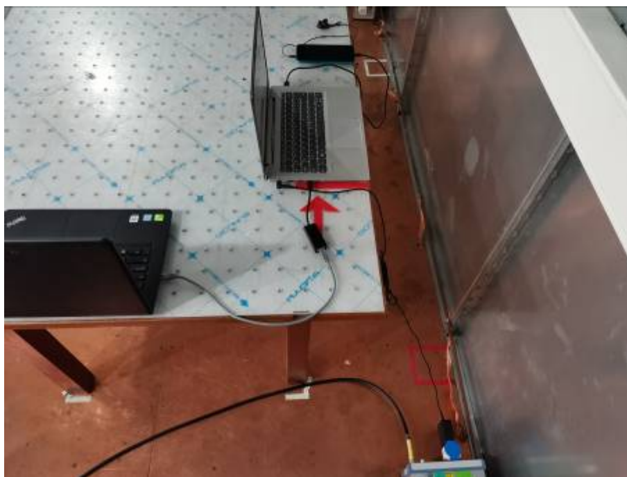
Conducted Emissions Test Setup
