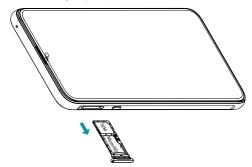
To eject SIM or MicroSD cards, insert your SIM eject pin into the small hole next to the card tray.
