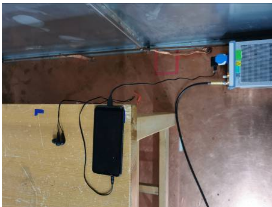
Conducted Emissions Test Setup (with charger)
