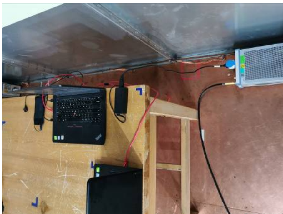
Conducted Emissions Test Setup (with laptop)
