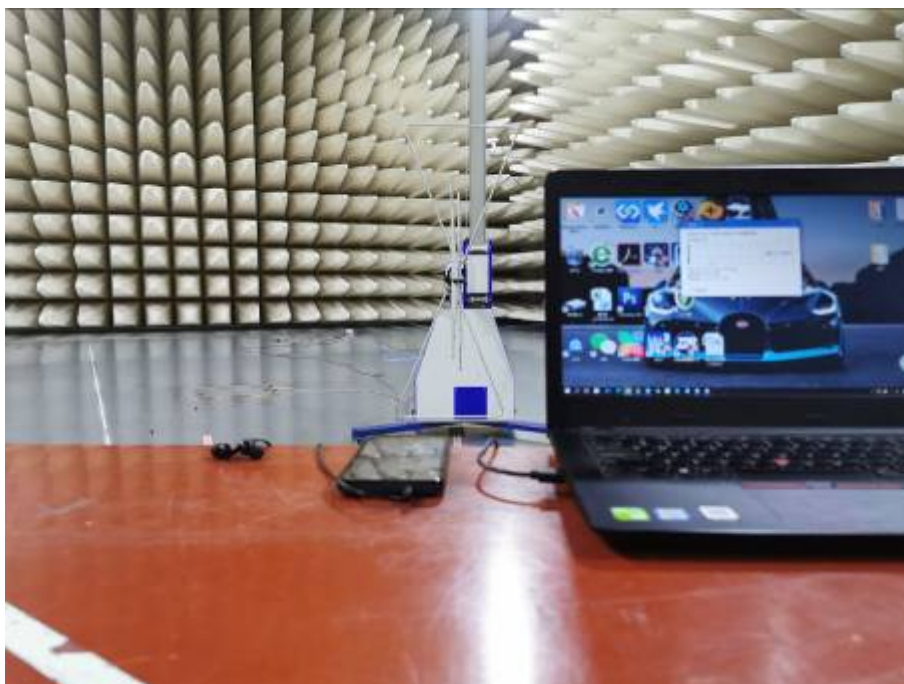
Radiated Emissions Test Setup (with laptop) (30-1000MHz)
