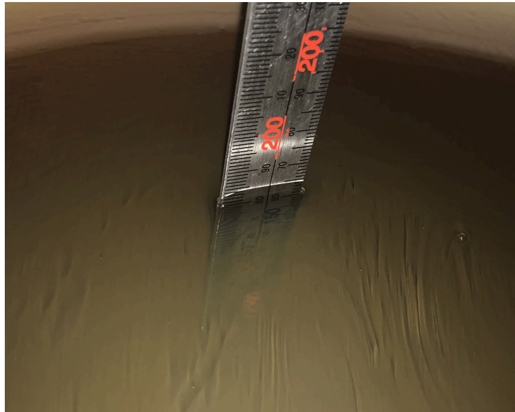
Liquid depth for SAR Measurement
