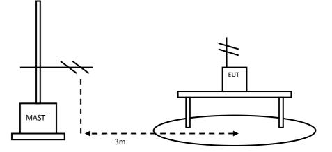
The Equipment Under Test (EUT) was set up on a non-conductive table in the semi-anechoic chamber. The test was performed at the distance of 3 m between the EUT and the receiving antenna. The radiated emissions measurements were made in a typical installation configuration. Then start the test software ES-K1. Sweep the whole frequency band through the range from 30MHz to 1GHz or above, using receive log period antenna HL562 or Ridge horn antenna HF906.
