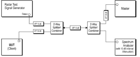
Setup of EUT CLIENT MODE:
