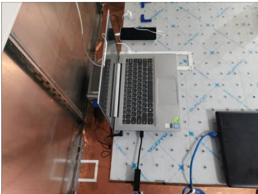
Conducted Emissions Test Setup (with laptop)
