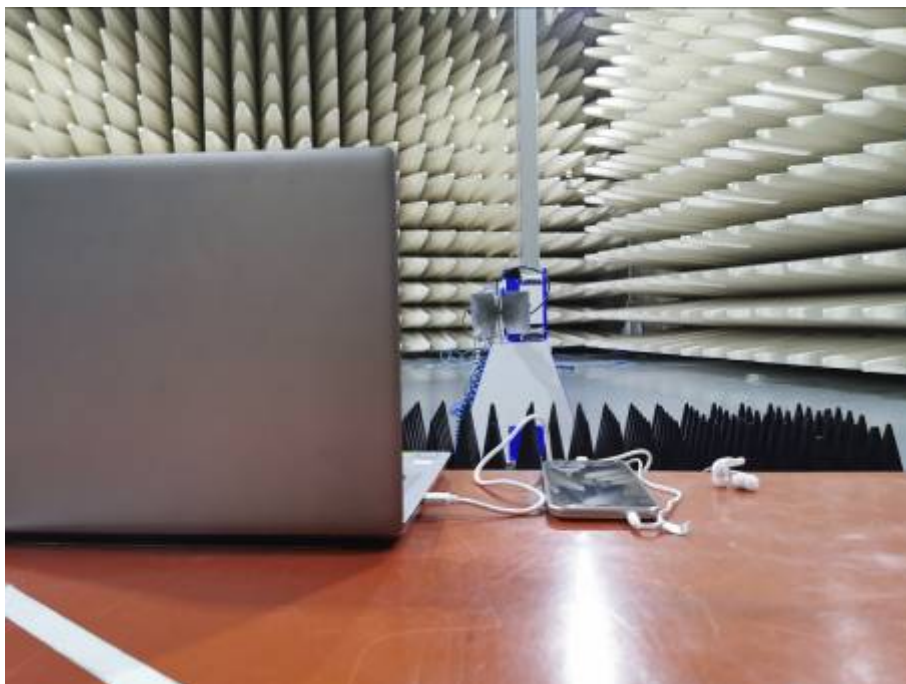
Radiated Emissions Test Setup (with laptop) (above 1GHz)
