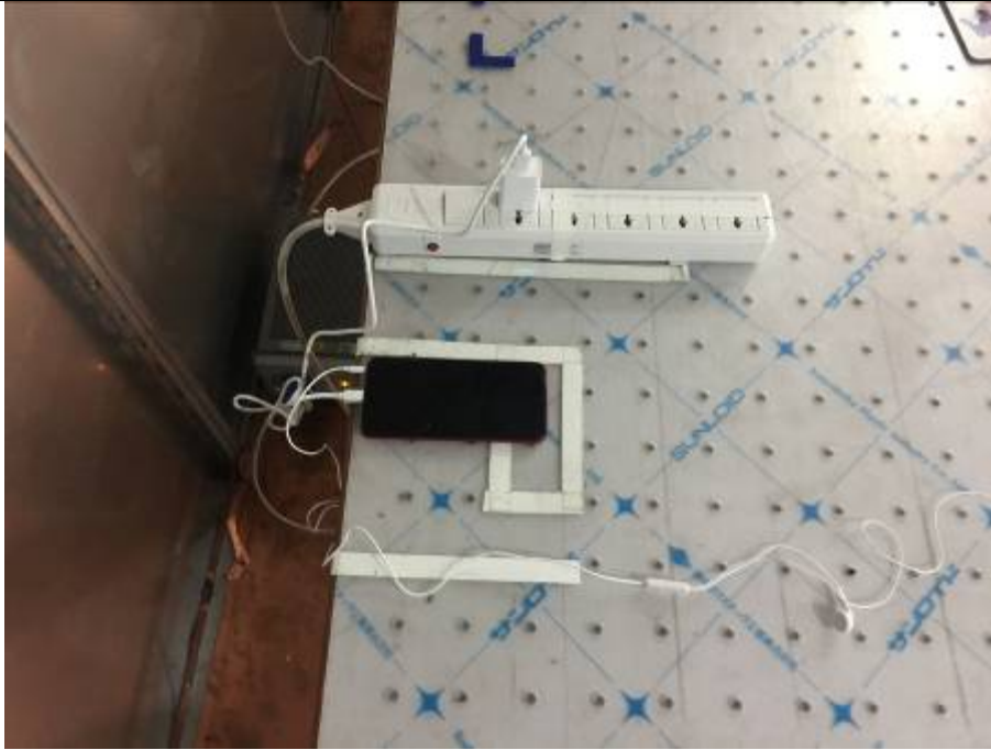
Conducted Emissions Test Setup (with charger)
