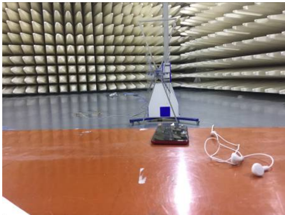
Spurious Radiated Emissions Test setup
