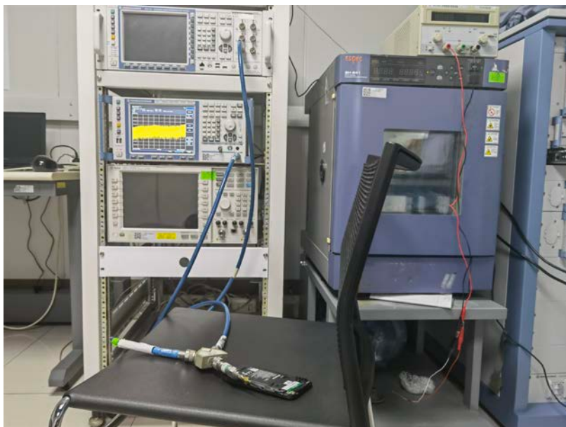
RF Conducted Test setup (GSM/WCDMA/LTE)
