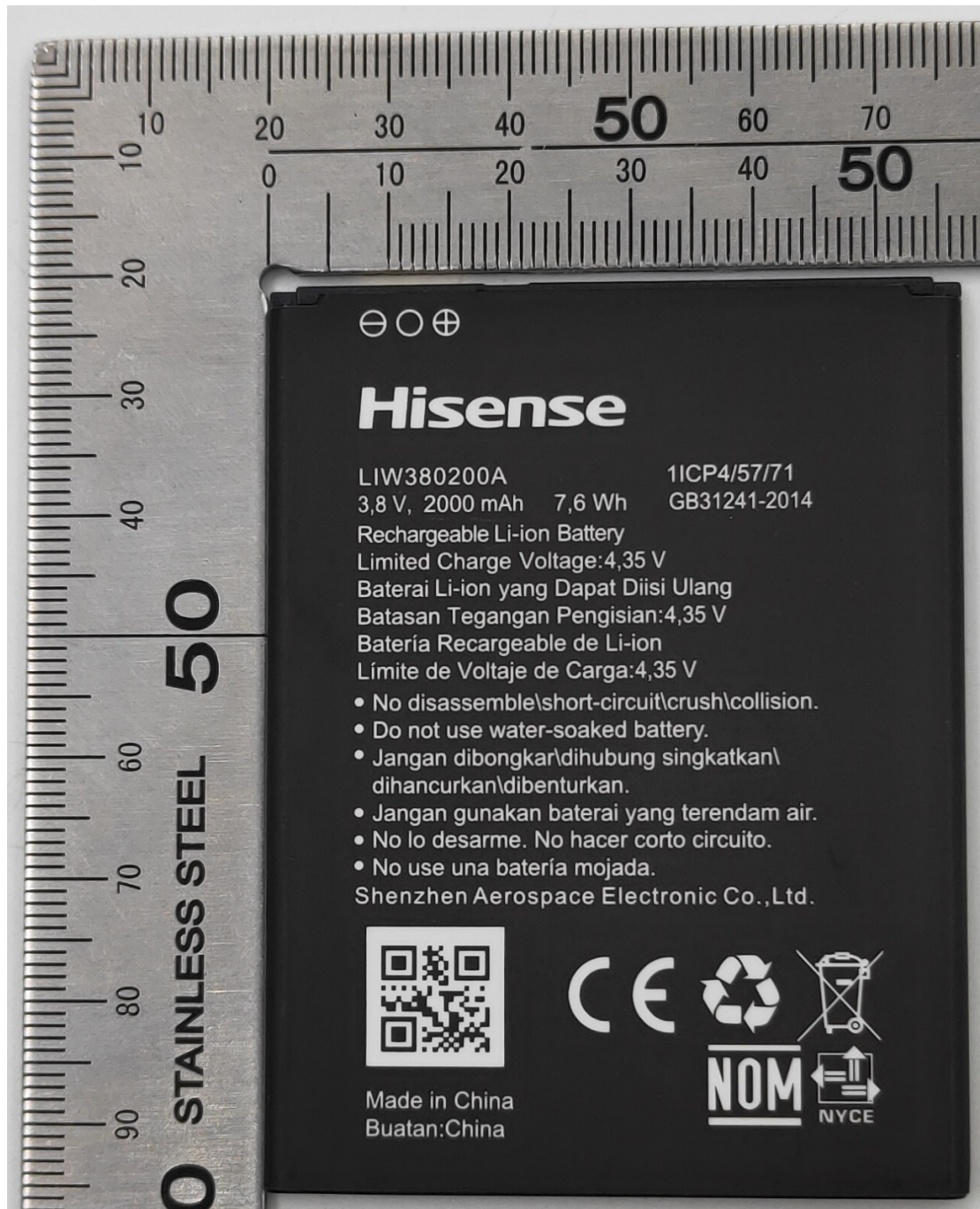
The battery view (ShenzhenAerospaceElectronicCo., Ltd.)
