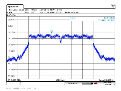
Carrier frequency (MHz): 2437 Channel No.6 Test Mode: 802.11n (HT20)
