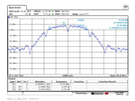
Carrier frequency (MHz): 2437 Channel No.:6 Test Mode: 802.11b
