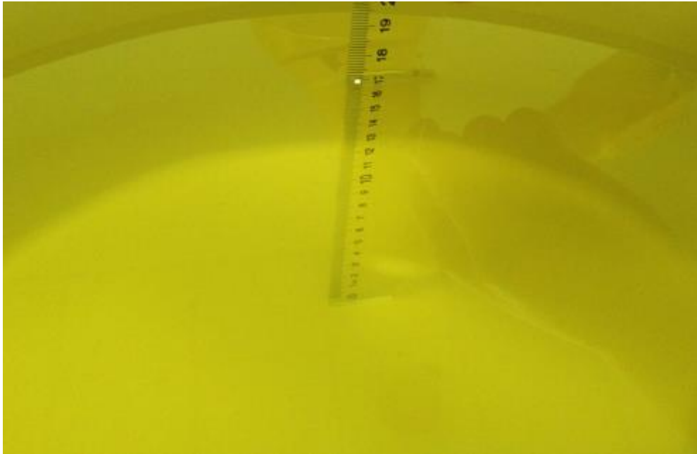
Picture 7-2: Liquid depth in the Flat Phantom (1900 MHz Head)
