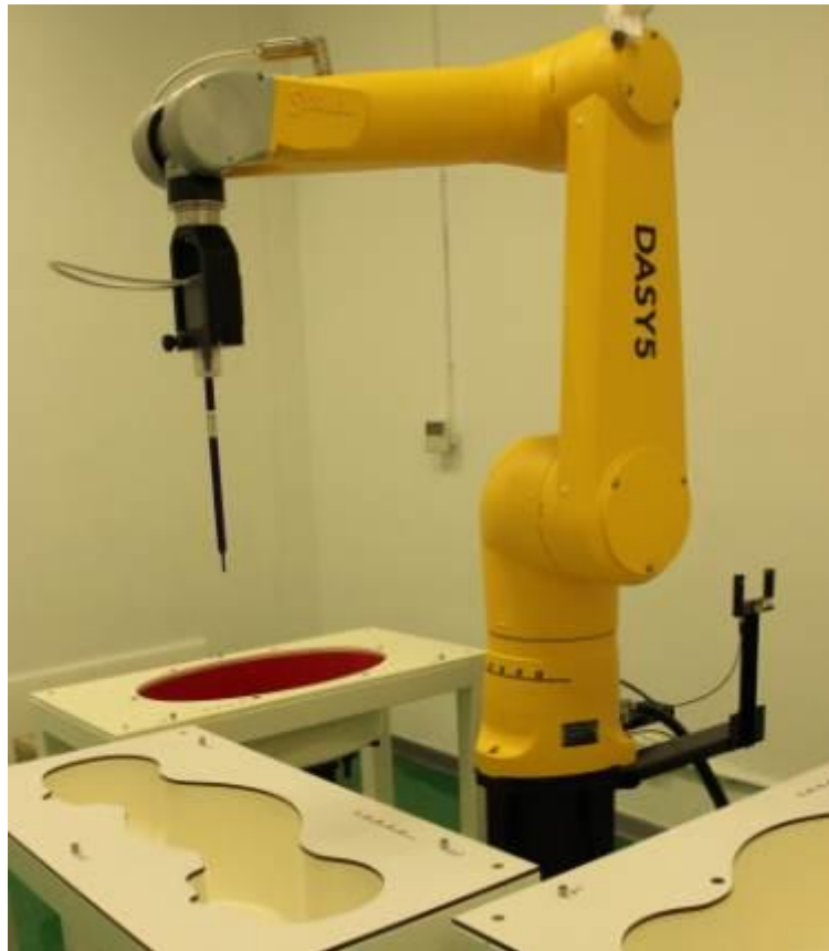
Picture D.6 DSY5 system Set-up
