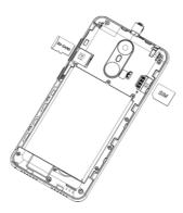
Ensure that the card is correctly aligned and that the card tray is level when you insert it into your device.
