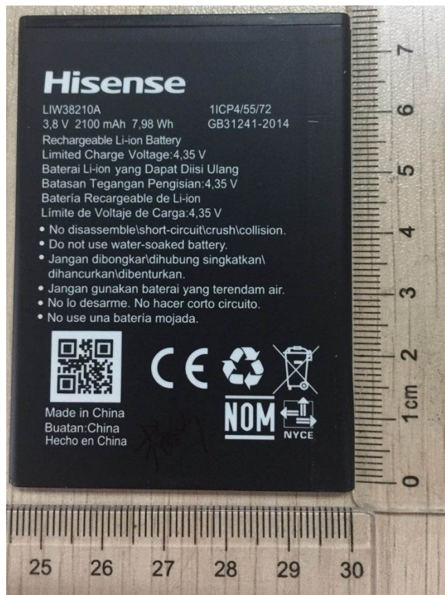
The battery view (LIW38210A Made by Guangdong Teamgiant New Energy Tech Co.,LTD.)
