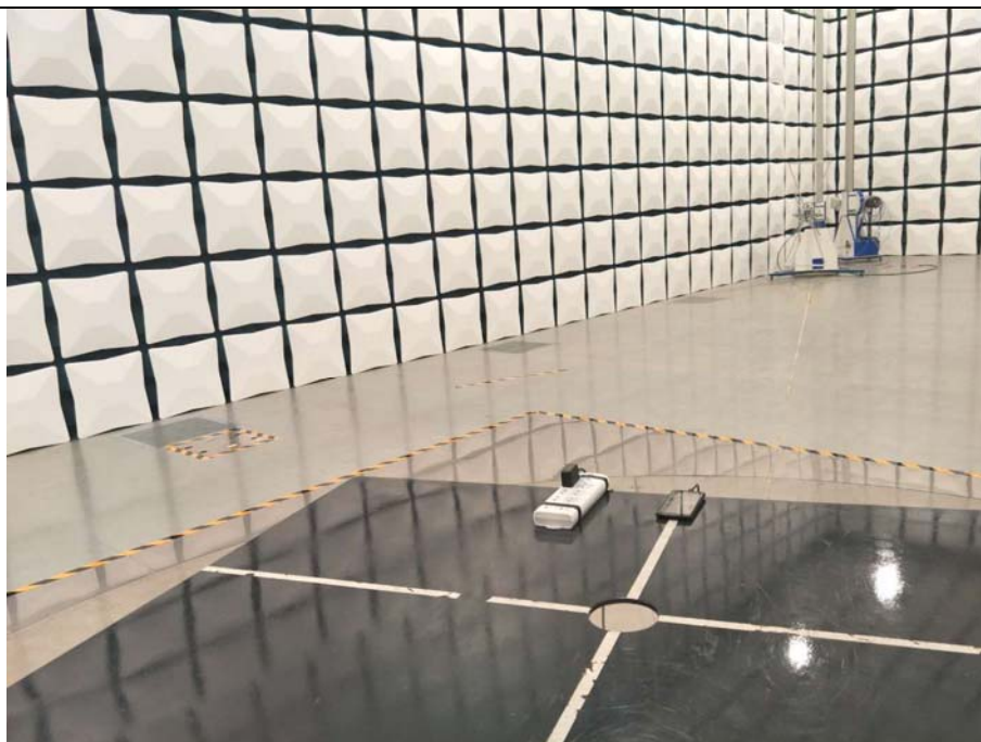
Spurious Radiated Emissions Test setup (below 1GHz)
