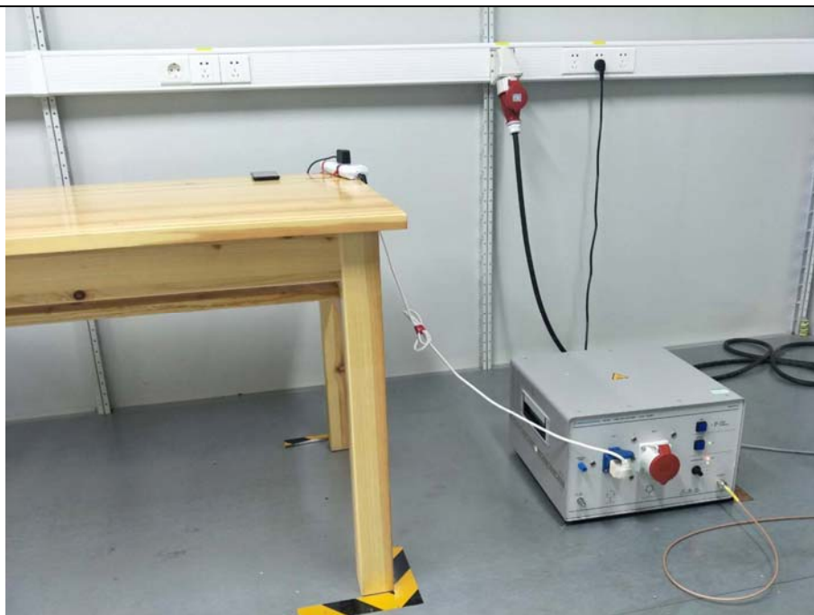
Conducted Emissions Test Setup (with charger)
