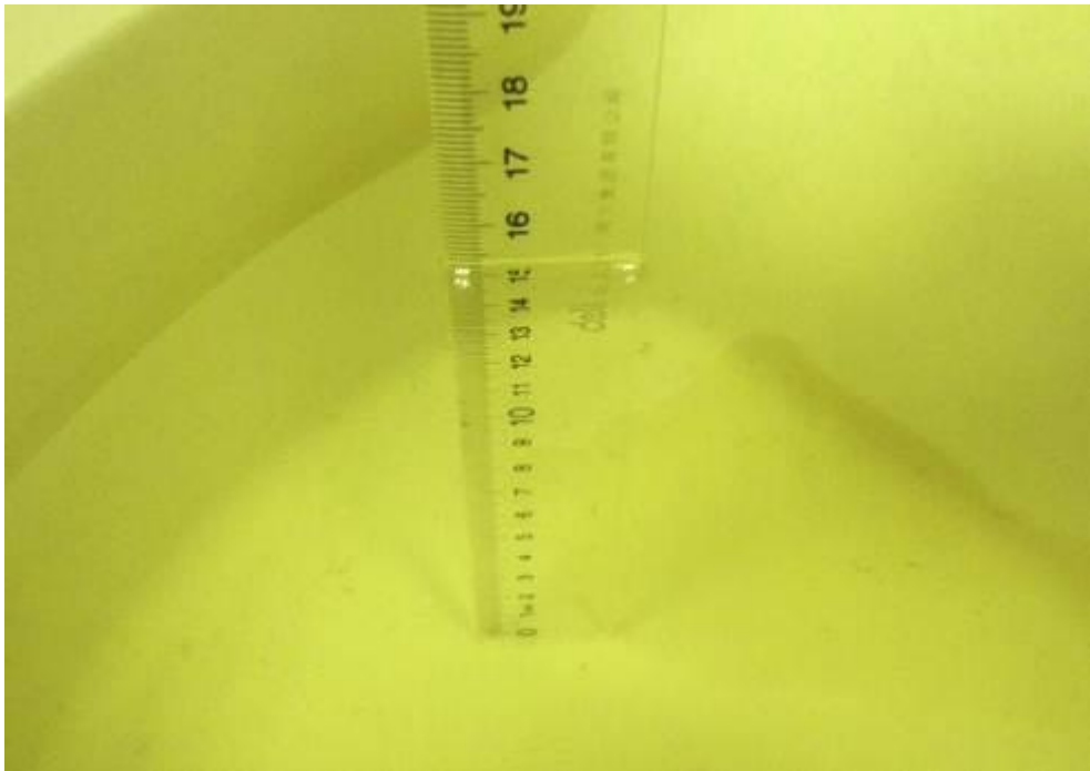
Picture 7-4: Liquid depth in the Flat Phantom (1900 MHz Body)
