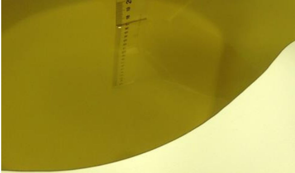
Picture 7-1: Liquid depth in the Flat Phantom (835 MHz Head)
