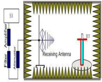
2. The EUT is then put into continuously transmitting mode at its maximum power level during the test. And the maximum value of the receiver should be recorded as (Pr).
