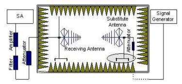
In the chamber, an substitution antenna for the frequency band of interest is placed at the
