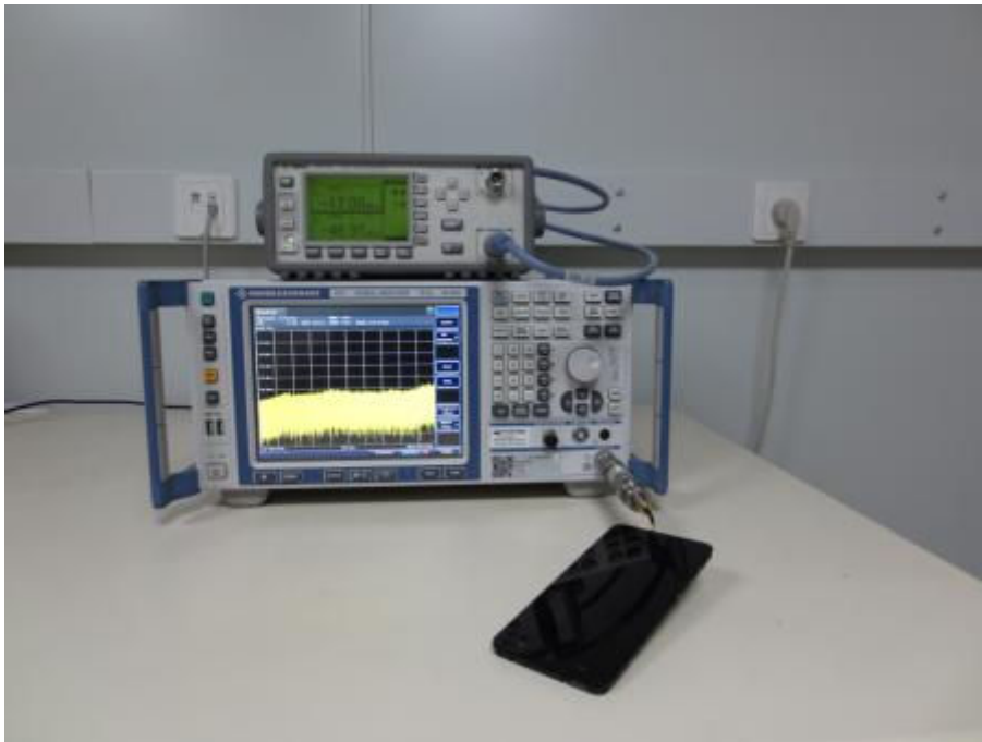
Spurious RF Conducted Emissions Test setup
