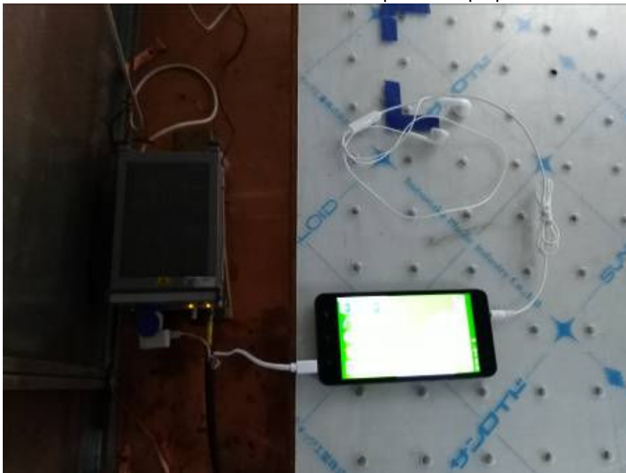
Conducted Emissions Test Setup (with charger)
