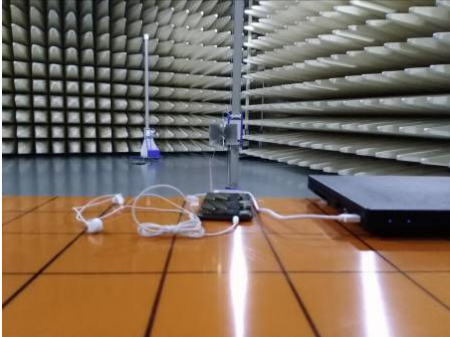
Radiated Emissions Test Setup (with laptop)
