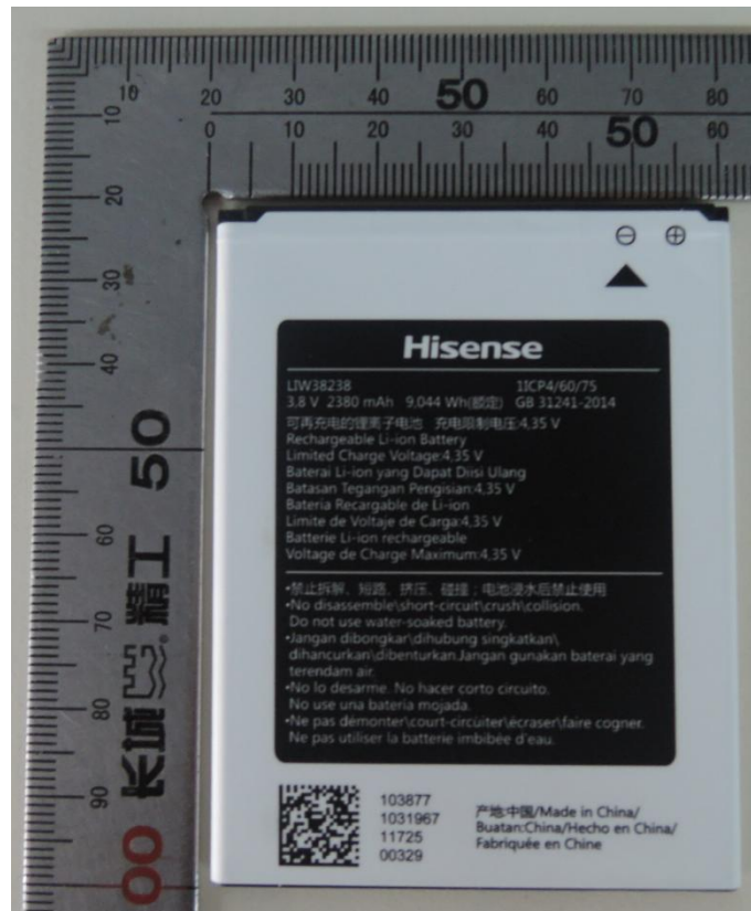
The battery view (Li3822T43P3h716043)
