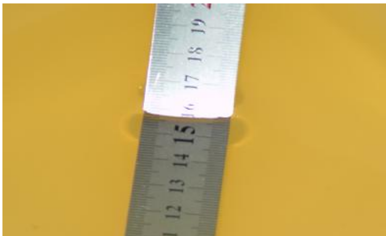
Liquid depth for SAR Measurement
