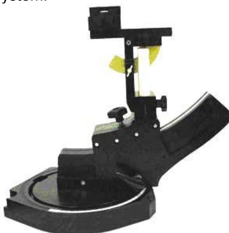
Device holder supplied by SPEAG
