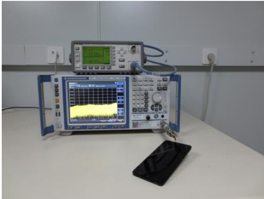
Spurious RF Conducted Emissions Test setup
