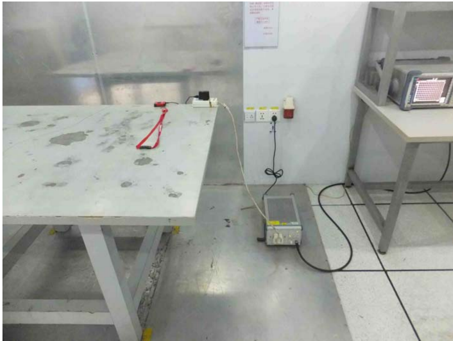
1 Photo of Power Line Conducted Emission Measurement
