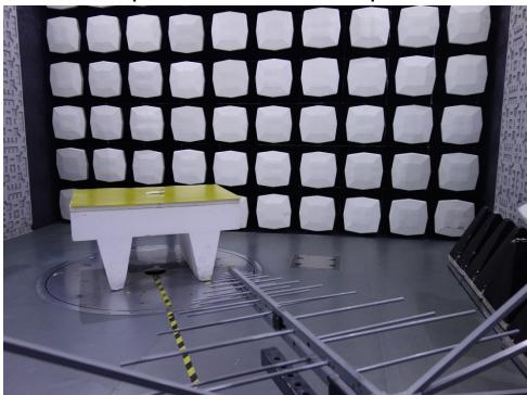
2.2 Radiated Spurious Emissions Test Setup
