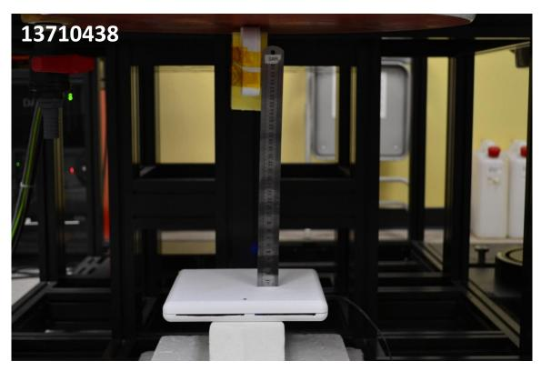
DUT is 26cm from the client device. The client device is 9 cm long giving a total DUT to phantom separation distance of 35 cm.
