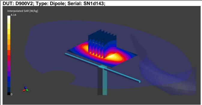
Communication System: CW UID: 0; Frequency: 900.0 MHz; Duty Cycle: 1;
