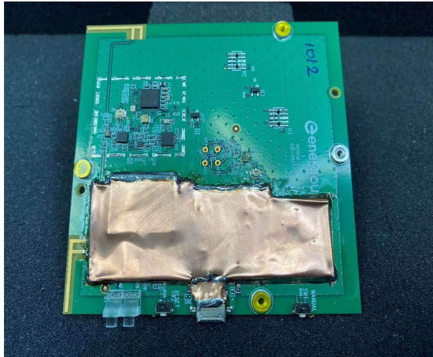
PCB Top View with Shield
