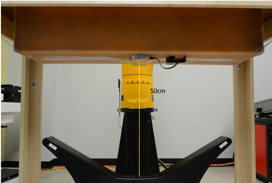
DUT located under Phantom (0 degrees, 50cm with watch connected to client device)
