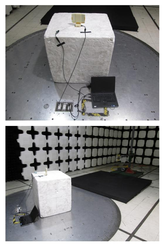
Radiated Emissions Test Configuration Photographs
