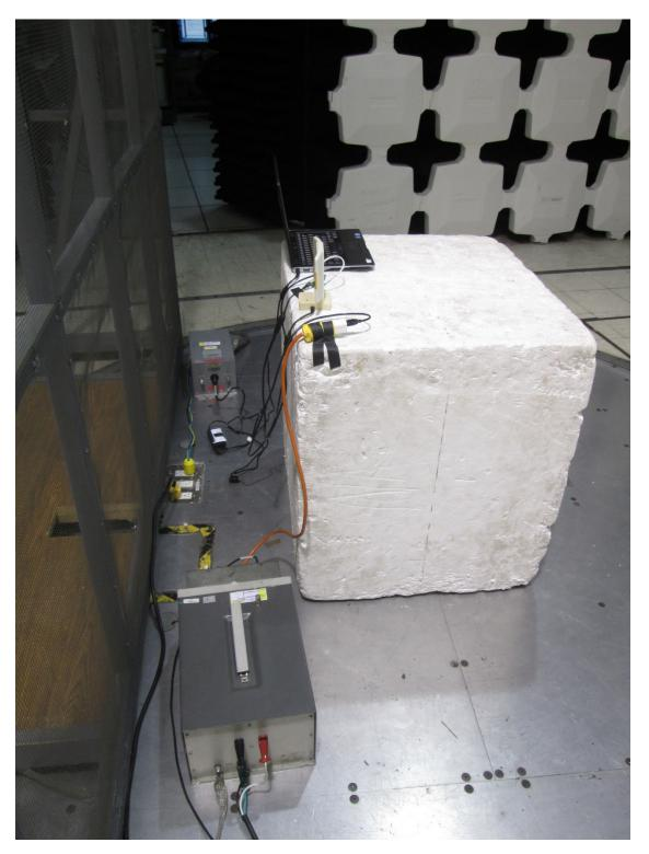
Conducted Emissions Test Configuration Photographs
