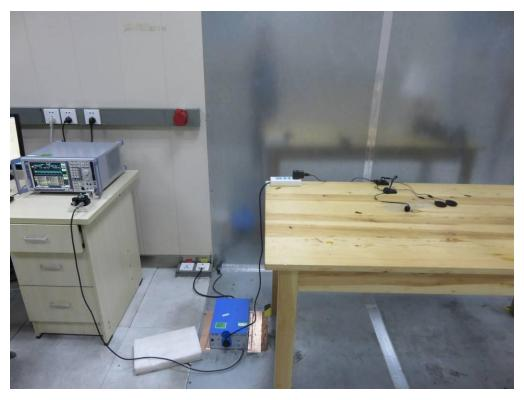
FCC RADIATED EMISSION TEST SETUP
