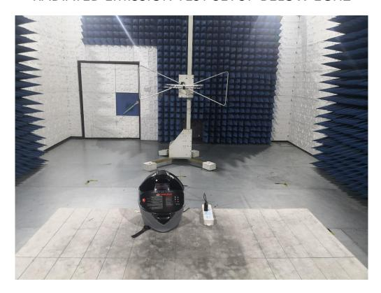
RADIATED EMISSION TEST SETUP ABOVE 1GHZ
